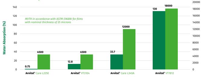
A key measurement of breathability is the Moisture Vapor Transmission Rate (MVTR) – a test that assesses material permeability to water vapor. Requirements for MVTR, water absorption, gas permeation to oxygen, and membrane flexibility and softness vary from application to application. Thanks to Arnitel Care and Arnitel VT's versatile chemistry, membranes can be designed to meet a wide range of property requirements that can't be achieved through microporous membranes.
