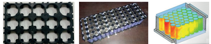
Figure 6: Passive battery cooling with battery tray made of conductive plastics (left). Battery specific thermal analysis to identify the impact of hot spots (right).
