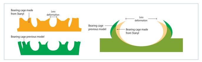
Fig. 6. The switch to Envalior's PA46 Stanyl allows lower deformation due to centrifugal forces in the SKF cages. © Envalior
