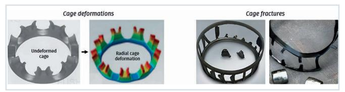
Fig. 3. Cage deformations (left) and cage failures (right) are caused by high rotational speeds and centrifugal loads, among other things. © Envalior
