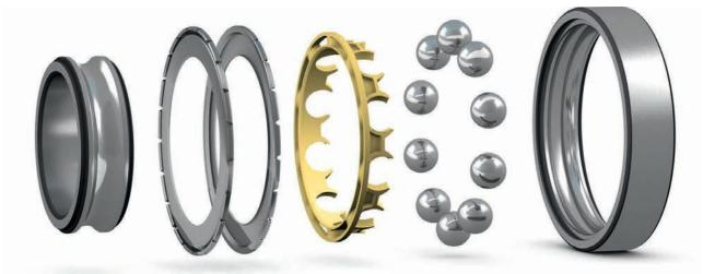
Fig. 2. SKF deep groove ball bearings using a polymer cage: The plastic bearing cage holds the rolling elements in the correct position. It must be resistant to mechanical and chemical stresses and ensure low friction. © SKF
