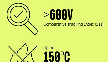
Relative temperature index (RTI) at 0.4mm thickness
