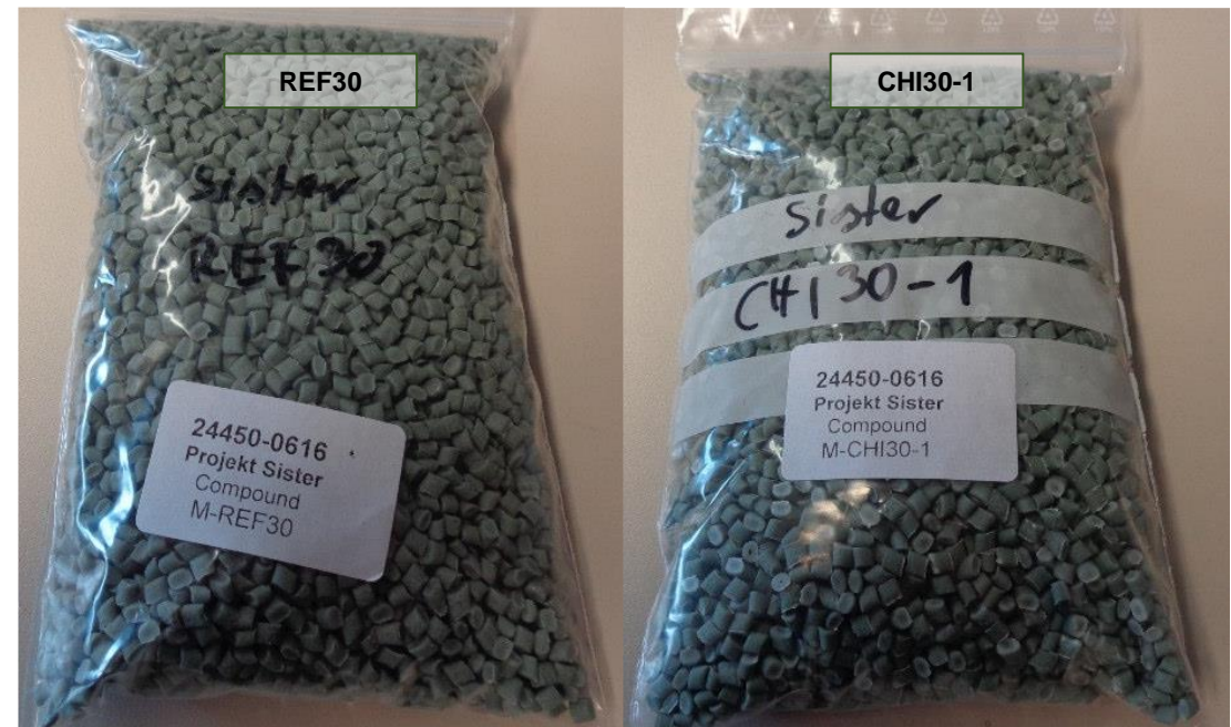
Figure: Comparison of the 30 wt.% compounds REF30 (reference) and CHI30-1 (sample)
