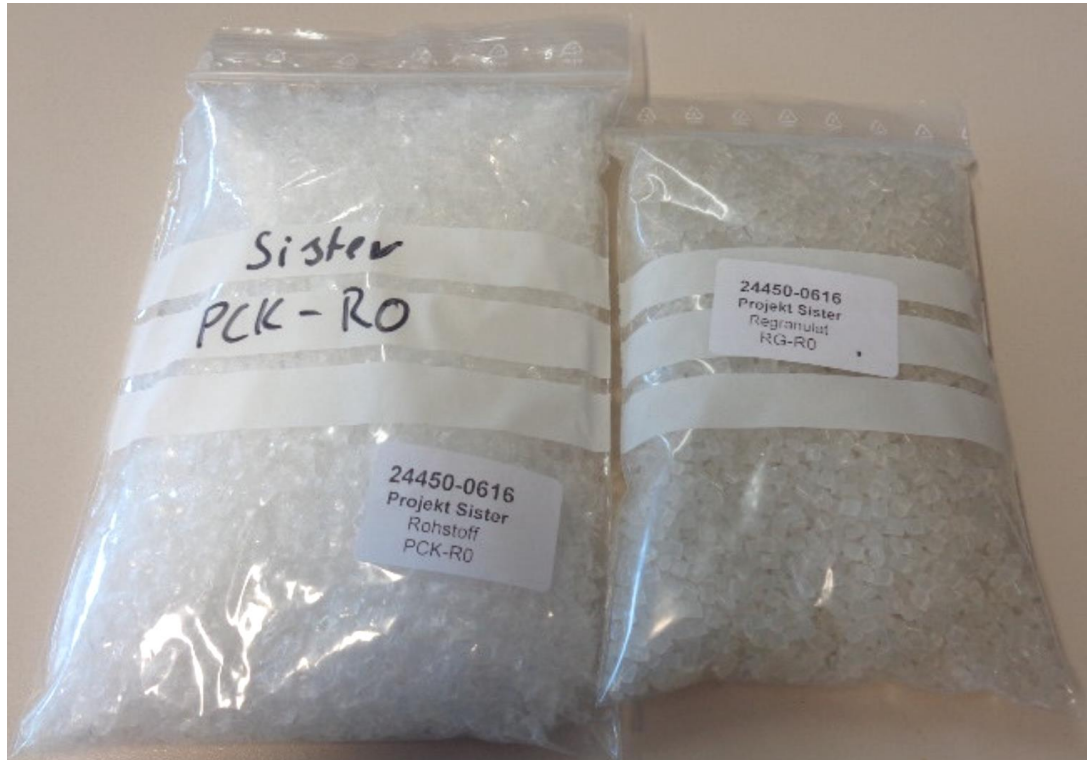
Figure: Flakes (left) and regranulate (right) of PCK-R0 (PE-reference without PA).
