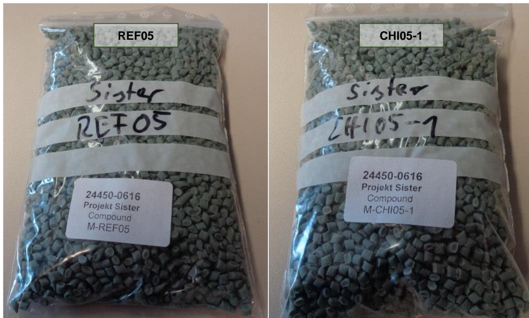
Figure: Comparison of the 5 wt.% compounds REF05 (reference) and CHI05-1 (sample)
