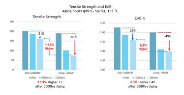
Xytron G4080HR's bonding interface technology also improves tensile strength and EAB at weld lines. Widely regarded as the weakest links in the structure of a part, weld lines inevitably appear on TMS parts during injection molding. The weld lines' tensile strength also determines the strength of the entire part, and therefore the part thickness required to meet the application's requirements.
