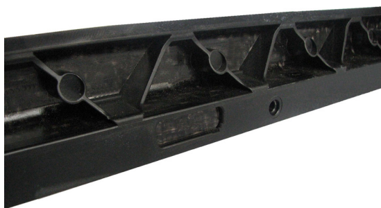
Figure 25: Example showing rib structure and injection-molded edges
