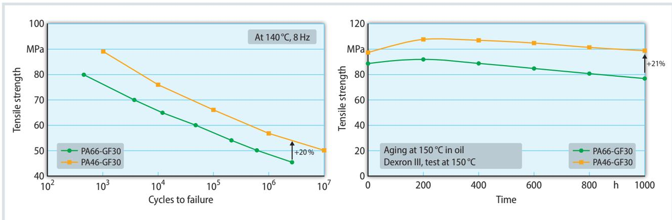
**Fig. 5.** Fatigue strength (left) and strength retention after exposure to 150°C hot oil (right) for glass fiber-reinforced PA66 and PA46. PA46 performs better in both cases. Source: Envalior; graphic: © Hanser
