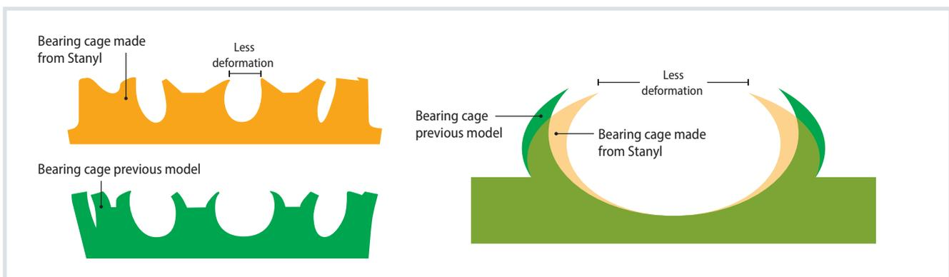
**Fig. 6.** The switch to Envalior's PA46 Stanyl allows lower deformation due to centrifugal forces in the SKF cages. © Envalior
