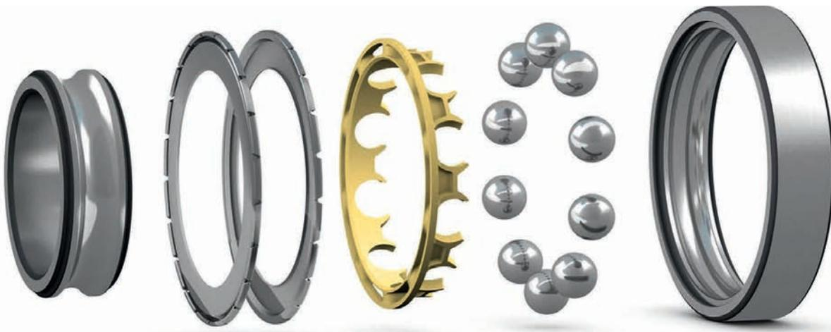
**Fig. 2.** SKF deep groove ball bearings using a polymer cage: The plastic bearing cage holds the rolling elements in the correct position. It must be resistant to mechanical and chemical stresses and ensure low friction. © SKF
