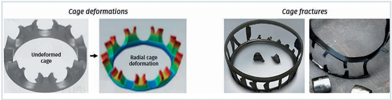
Fig. 3. Cage deformations (left) and cage failures (right) are caused by high rotational speeds and centrifugal loads, among other things. © Envalior
