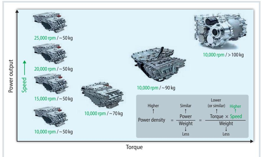
Fig. 7. Higher motor speeds increase the power output and power density of electric motors.
